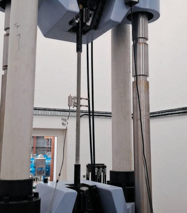
UTM performing tensile testing of Mateenbar™
