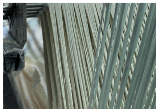
Epoxy vinyl ester resin during pultrusion process
