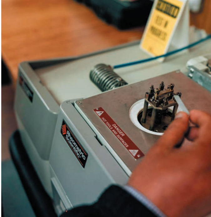
DMTA testing to ensure full cure of Mateenbar™
